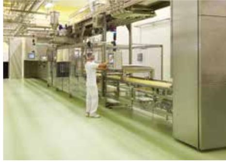
(Below) The new moulding lines are capable of running bars at a rate of 30 moulds per minute.
